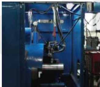
Plasma spray plus automatic powder feeding use for oil drill pole
