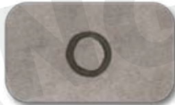
INVERTER SPOT STAINLESS STEEL 2+2 MM
